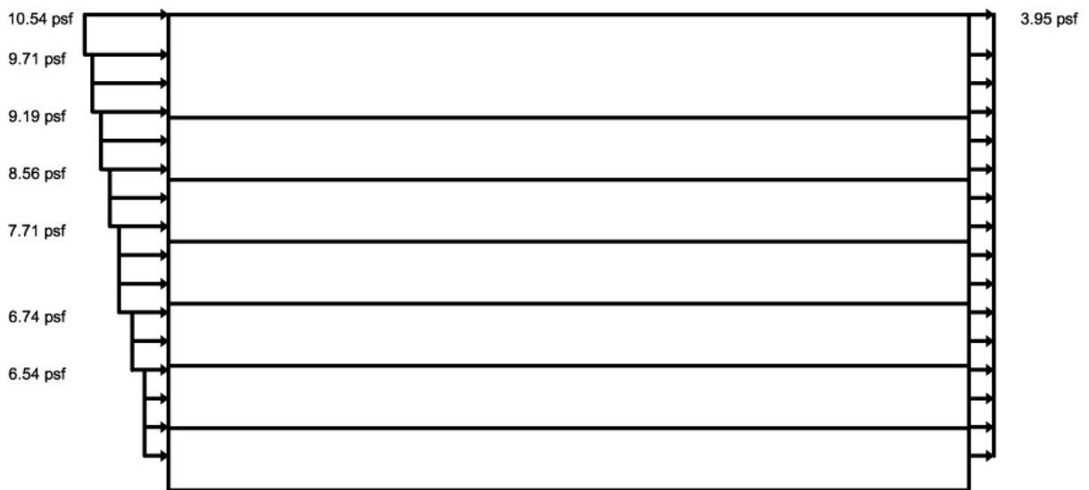
Figure 4: North Building Wind Pressure Diagram in the North – South Direction
