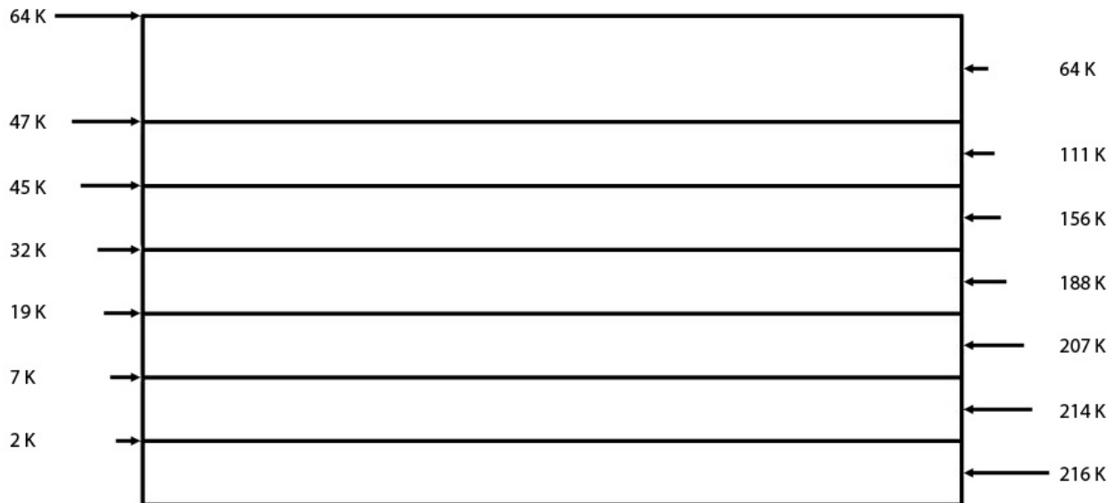
Figure 6: NWC Braced Frame Building Seismic Force Diagram
